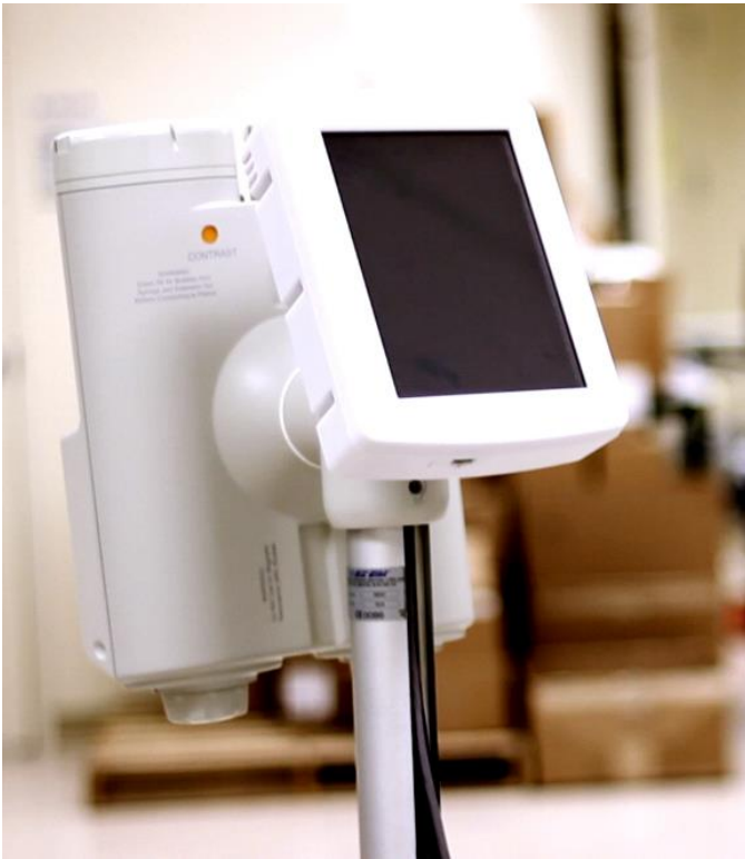
This screen housing from Acist Medical was 3D printed with production-grade ABS.
