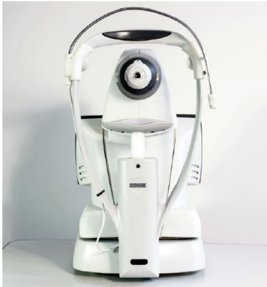
The assembled Gonioscope® prototype, built with 3D printed parts.
