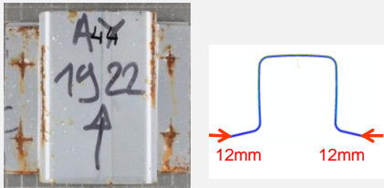
E-coated omega After corrosion
