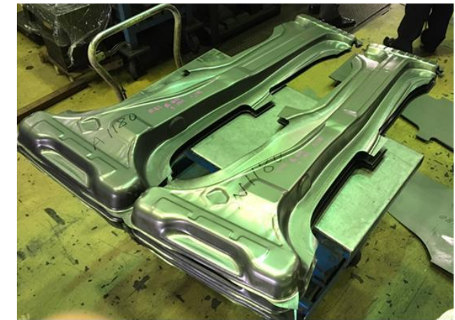
Fortiform®1180 bare 1,2 mm Reinforcement B-pillar trial
