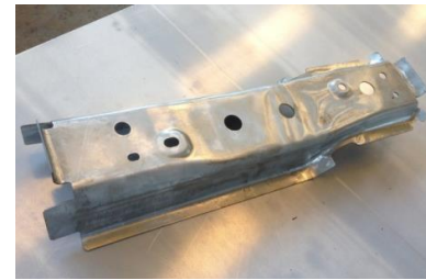
Fortiform®1050 EG 1.3 mm Reinforcement Seat Cross Member
