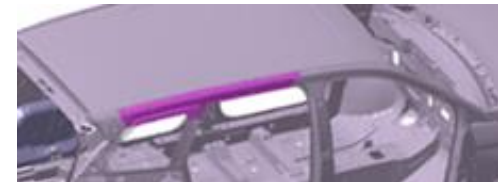
Fortiform®1050 bare 0,85 mm Reinforcement roof arch
