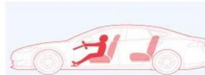
The vehicle can perform some driving functions, often with a single feature such as cruise control. The driver maintains control of the vehicle.
