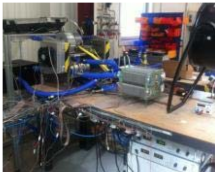
10kW stack with Liten MEAs operating in a system
